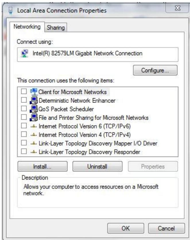
Click on the check boxes to remove the check marks from all the protocols that the connection uses. This will prevent Windows from trying to access the Internet or a Windows network over this port.
