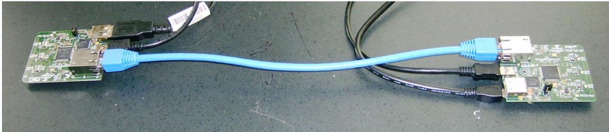
To use the SharkTap to monitor the Ethernet packets on that link, connect the SharkTap as shown in the next picture:
