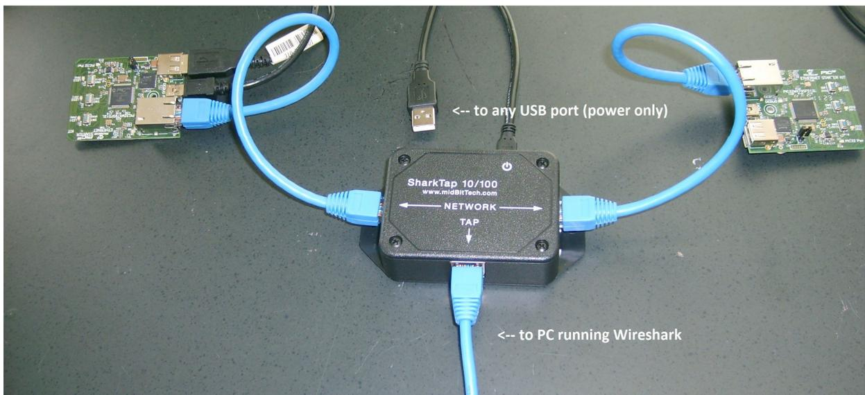
The two Ethernet devices connect to the two side ports marked 'NETWORK'. All packets on either network port will be duplicated on the TAP port. The TAP port is typically connected to a PC running the Wireshark analyzer. Finally, connect the USB cable from the back port to any USB port, or use any cell phone charger with a micro-USB connector. The red LED on the back will light red to show power is attached. (The SharkTap will not show up as a device when connected to a PC, it only draws power)
